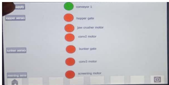
Fig 15 : HMI screen showing ON state of conveyor-1
