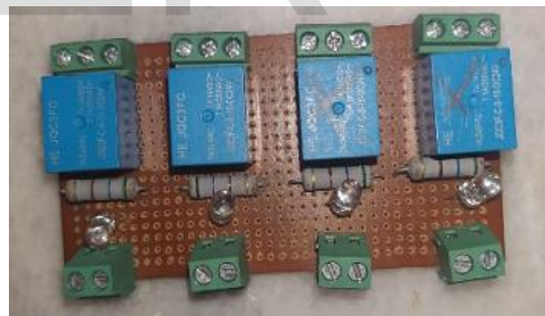
Figure 10 : 4 channel relay motor
